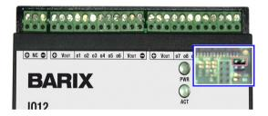
J3 is a 4 pin connector and is located next to LED1 and LED2. To set default parameters connect the upper two pins using a standard jumper (not included).
