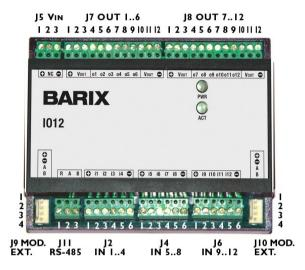
J5 Pin out V<sub>IN</sub> Power supply input of the BARIX IO12.
