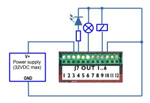
Both connector blocks (J7 and J8) must be powered either on Pin 1,2 or 3 and grounded either on Pin 10,11 or 12 in order to function correctly.
