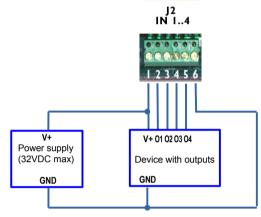
Each used connector block (J2,J4,J6) must be powered on Pin 1 and grounded on Pin 6 (as shown in picture above) in order to function correctly.
